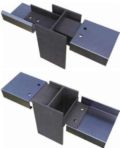
INTERIOR GIRT TO COLUMN CONNECTION DETAILS
