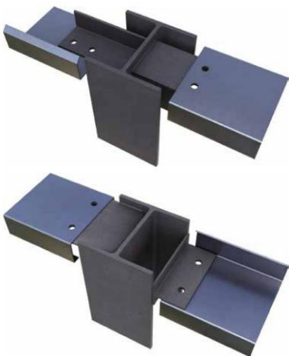
INTERIOR GIRT TO COLUMN CONNECTION DETAILS
